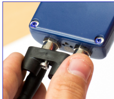
II. Remove Connectors Locking Clip (CLC)
