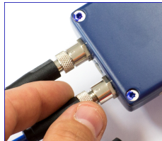
III. Manually unscrew connector of spare unit (for example cutter)
