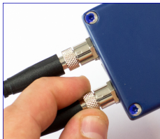
V. Reconnect and manually tighten the new spare unit (Cutter or Control unit)
