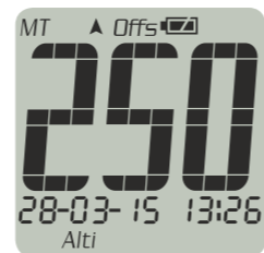
Ground mode with an offset set as landing zone at +250 m from take off place
