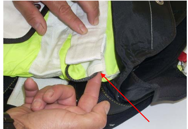
Tuck any excess RSL into the channel pocket on the top left side of the free-bag.
